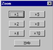
To magnify the graph horizontally, press "**Zoom**" and choose one of the possible magnifications (x2, x4, x5, x8, and x10). The chosen value is shown on the right side of the display window.
