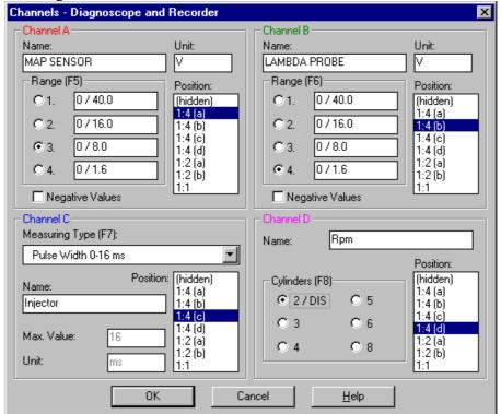
In **Channel C** you may change the type of measuring (see Universal Channel). When you press **[F7]** or **"Channels"**, you will see the list of types. There are available measurements of e.g.
