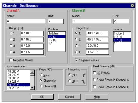
The "Synchronization" settings let you choose the channel, with which the displaying of the graphs should be synchronized, and the level, crossing of which should make drawing the graphs start. You may also choose if displaying should start from the increasing (INC) or decreasing (DEC) slope of the signal. You may regulate the voltage of displaying (level of synchronization) directly in the main window of Diagnoskop. To do this, you should move the
