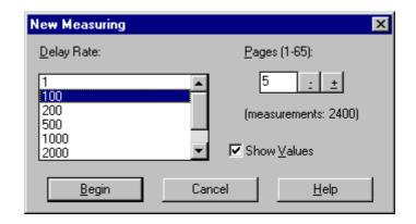
The program counts the delay for "recorder" and "diagnoskop" modes in a form of measurements that are skipped.
