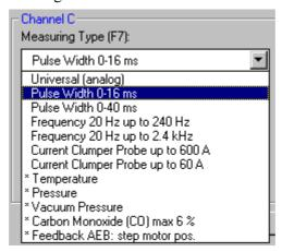
In **Channel C** you can make the measurements of:
