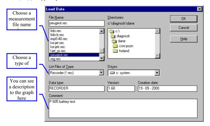
Notice that there are additional elements in the shown window. If you point some file, the program will automatically recognize its version and type. If you added the comment to the data during the saving process, it will be also shown. In this way you may easily and quickly find the interesting file.
