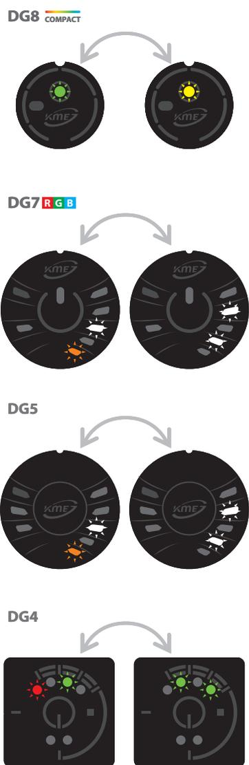
1. Turn the ignition on (the autogas tank must be empty).
