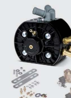
Reducer is intended to be used in engines that are characterized by **large temporary gas intake** in cars, where two reducers can be installed. **Resistant to dirt** in the gas. Every each side has their own pressure regulation. Version V1 with **TWO SOLENOID VALVES.**
