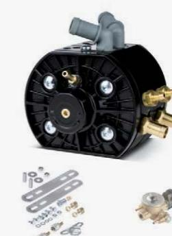
Reducer is intended to be used in engines that are characterized by **large temporary gas intake** in cars, where two reducers can be installed. **Resistant to dirt** in the gas. Every each side has their own pressure regulation. Version **V2** with **ONE SOLENOID VALVE** with **FARO** outlet.
