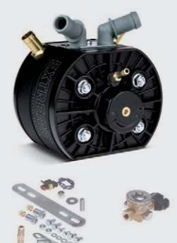
**Reducer designed for extreme tasks.** Additional heating module allows for use in high engine cars up to 408 HP. Increased flow sections allows to keep proper gas parameters.
