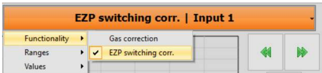
Fig. 2.90 turning on EZP correction
